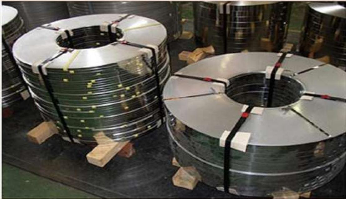
Type 304 Stainless Steel is the most widely used of the austenitic (chromium/nickel) stainless steels. In the annealed condition it is essentially non-magnetic and becomes slightly magnetic with the application of cold work. Type 304L Stainless Steel is preferred in welding applications to exclude the formation of chromium carbides during cooling in the heat affected region of the weld. These alloys represent an excellent combination of corrosion resistance and fabricability
