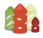
Coated foam pigs are used for regular wiping and general cleaning. Models are available in light, medium, and heavy density foam. The pigs are constructed from an open-cell polyurethane foam with a durable polyurethane elastomer coating in a variety of patterns with criss-cross being the most common.
